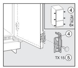
Screw bracket (4) using hex screw (5) to the pre-drilled holes in the appliance door. ■ Push the appliance two-thirds of the way into its niche.
